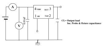
NB: Pin1 connected to VDD or floating, connect to ground stops oscillation
