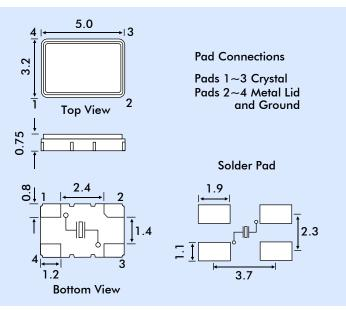
\* Note: These parts may be supplied with the chamfered pad in different positions. However, the crystal connection is always as shown above.
