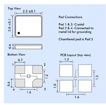
\* Note: These parts may be supplied with the chamfered pad in different positions. However, the crystal connection is always as shown above.
