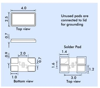
\* Note: These parts may be supplied with the chamfered pad in different positions. However, the crystal connection is always as shown above.
