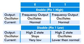
When Pad 1 is allowed to float it is held high by an internal pull-up resistor.
