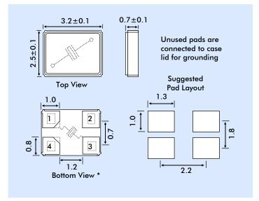
\* Pad Connections: Pad 1 and 3: Crystal Chamfered pad can be Nos.1 or 4
