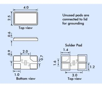
\* Note: These parts may be supplied with the chamfered pad in different positions. However, the crystal connection is always as shown above.
