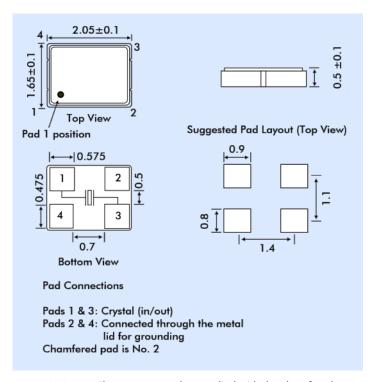
\* Note: These parts may be supplied with the chamfered pad in different positions. However, the crystal connection is always as shown above.
