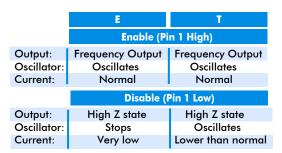
When Pad 1 is allowed to float it is held high by an internal pull-up resistor.
